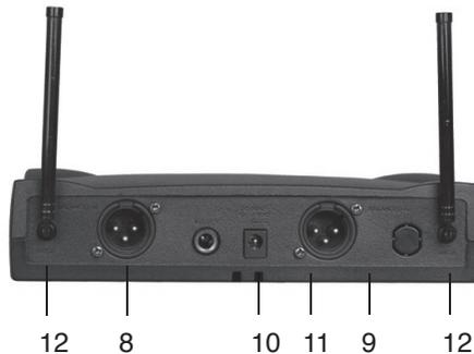
8. LINE OUT channel B: Unbalanced XLR line level output with audio signal from emitter B to connect a mixer, an amplifier or powered speaker cabinet.
