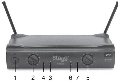
1. POWER switch: This switch turns on/off the power of the receiver.
